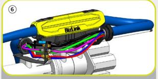
Detailed information for dresspack installation must be considered. During commissioning, ensure that the installation is free of collisions
